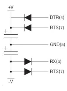
The TriStar uses an isolated "port powered" RS-232 connection, meaning that the circuitry uses a small amount of power from the PC that it is connected to.
