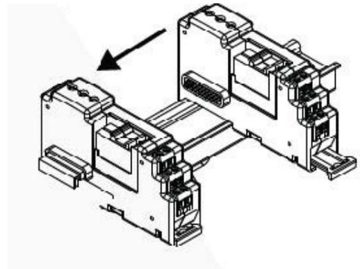
Blocks can be easily added to the ReadyRail standard DIN-mount and stacked to complete the system
